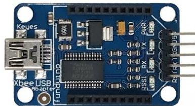
**Figura 2. 3 XBee USB Explorer [9]**
