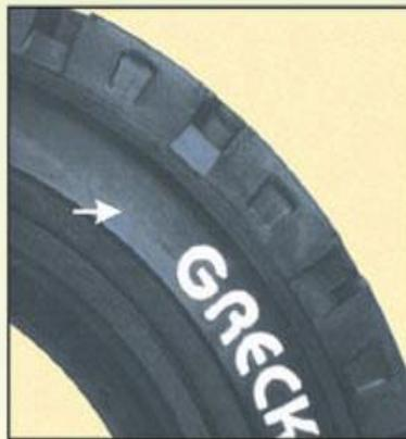
The mid Concave side wall design increases tyre deflection and reduces driver and equipment fatigue.
