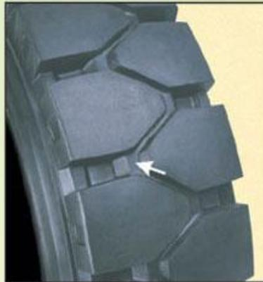
Center wear bar prevents tread shuffling during steering operations ensuring long and even treadwear and eliminates chipping and chunking
