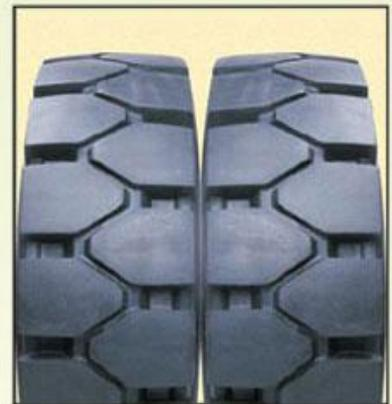
Wider footprint and large tread lugs help in reducing the strain on the tread thereby enhancing the mileage.
