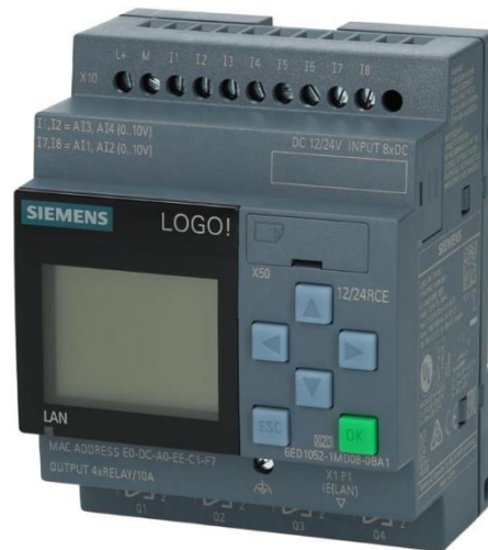
Figura 3.27 Micro PLC LOGO 8 de SIEMENS
