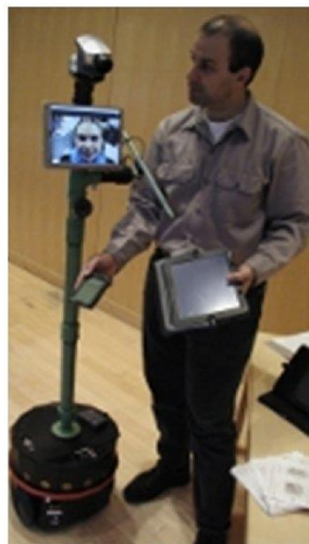
Figura 1.1 Tele-robot PRoP (Personal Roving Presences) [9]
