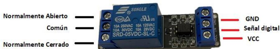
Figura 3.8 Relé SONGLE SRD-05VDC-SL-C
