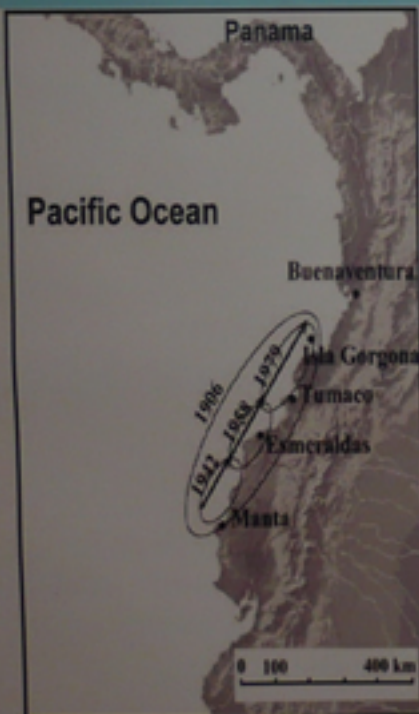
Figure 1. Direction of rupture propagation and rupture areas of large shallow earthquakes in the Ecuador-Colombia region (Keleher, 1972; Herd et al., 1981; Beck and Ruff, 1984).
