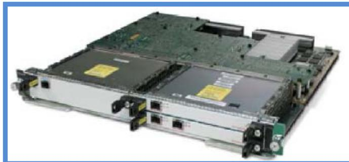
**Figura 3.46.- Tarjeta SPA Interface Processor.**
