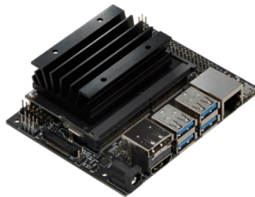
Figura 1.2 Jetson Nano Developer Kit [43]
