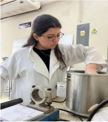
**Figura 2. 15***Pesaje en balanza de flotabilidad.*
