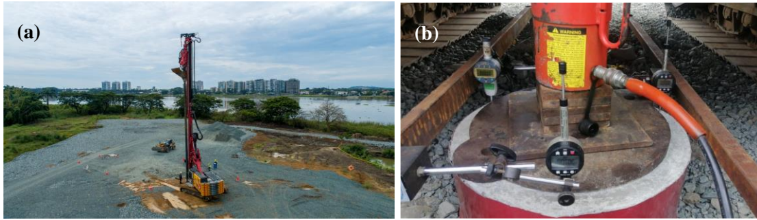
236 Figure 3. Configuration of a load test for the RAP during the study phase, Northern WWTP: (a) view
