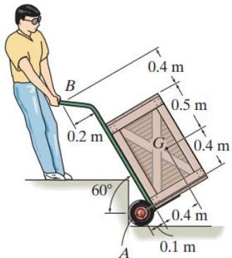
**Equations of Equilibrium.**  $P_y$  can be determined directly by writing the force equation of equilibrium along  $y$  axis by referring to the FBD of the hand truck shown in Fig. a.
