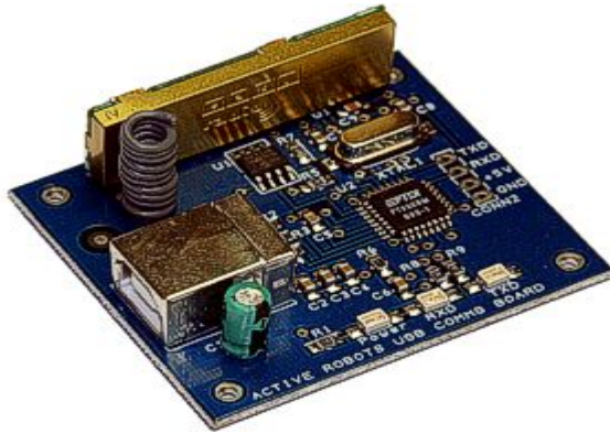
Figura 2.6 Radio modem usb 19.2Kb easy radio 433Mhz
