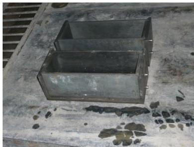
**FIGURA 4.12 Moldes metálicos viguetas de 100x100x285mm**
