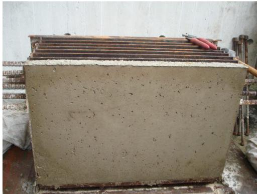
**FIGURA 5.6 Desmolde de paneles**
